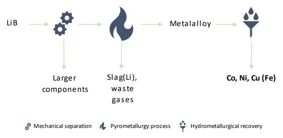
Figure 2 - Pyrometallurgical recycling simplified process flow diagram
