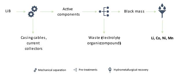
Figure 3 - Hydrometallurgical recycling simplified process flow diagram
