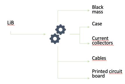
Figure 1 - Mechanical recycling simplified process flow diagram
