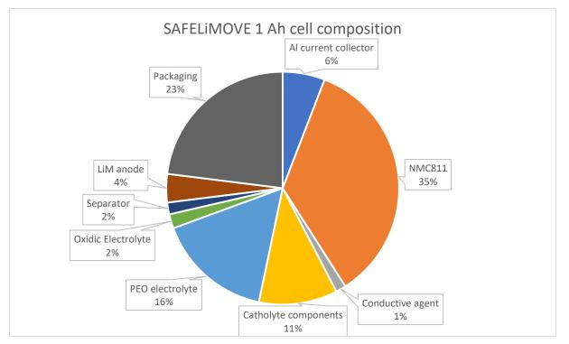
Figure 5 - SAFELiMOVE 1 Ah cell composition
