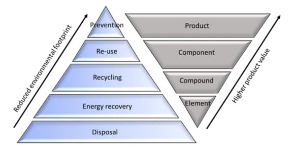
Lansinks Ladder according to the Council Directive 75/442/EEC representing the waste management hierarchy and the correspondence of product value levels to recycling.
