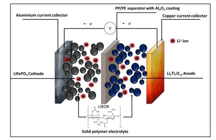
Lithium-ion battery cell design for improved safety and long lifetime
