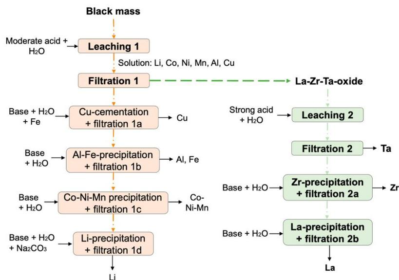
Figure 4 - Proposed hydrometallurgical recycling path for solid state battery (12)
