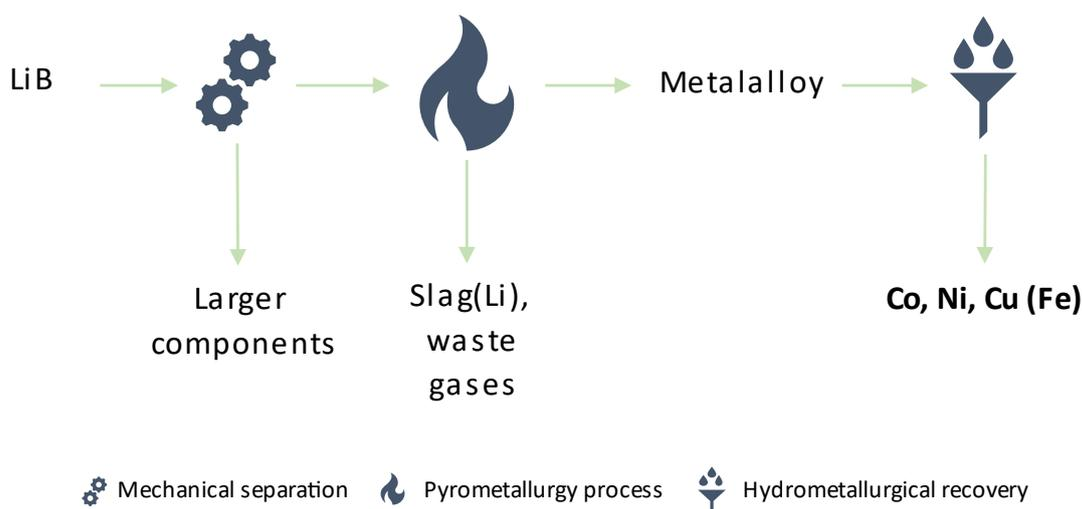
Figure 2 - Pyrometallurgical recycling simplified process flow diagram
