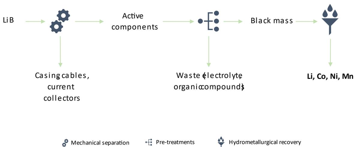
Figure 3 - Hydrometallurgical recycling simplified process flow diagram
